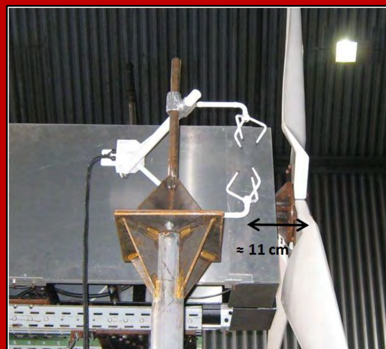
Figure 3: Three component sonic anemometer and blade orientation showing typical clearance.
