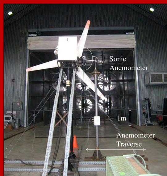
Figure 2: Anemometer traverse and wind turbine (looking upstream)
