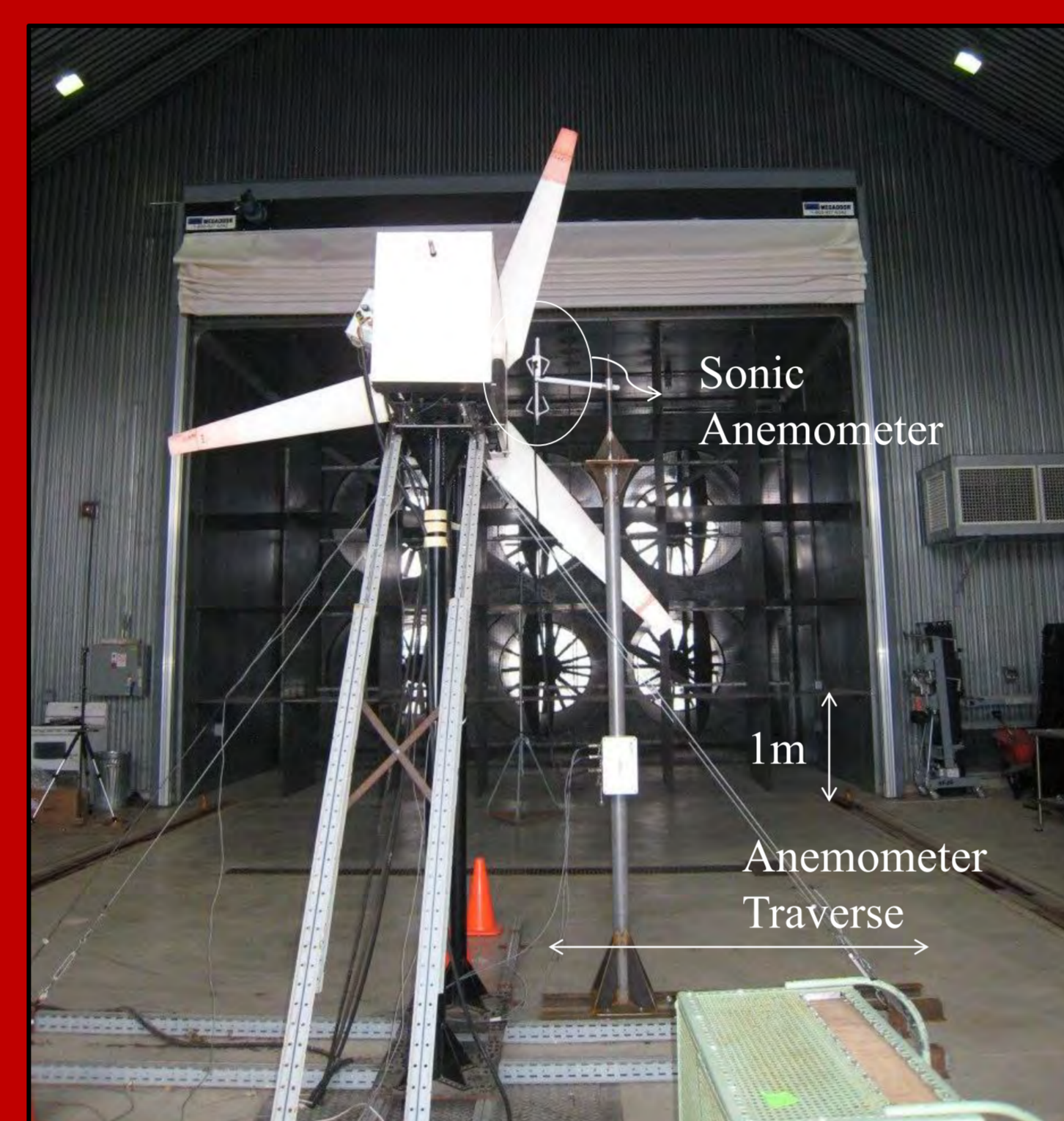
Figure 2: Anemometer traverse and wind turbine (looking upstream)
